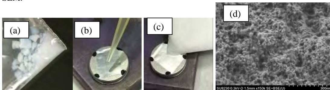
Fig. 1 Aerogel sample preparation and SEM image taken by SU8230 FE-SEM
